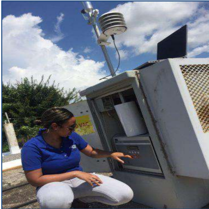
Acting Manager of the Air Quality Management Branch at the National Environment and Planning Agency (NEPA), Shannen Suckra, services a BAM1020 particulate analyser at NEPA's Spanish Town air quality monitoring station. When the concentration of PM2.5 is found to be higher than the World Health Organization's guideline, NEPA
