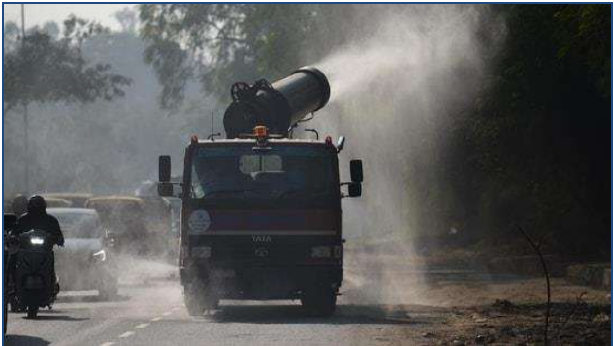
A truck mounted with an anti-smog gun is being used to spray water droplets to curb air pollution in New Delhi
